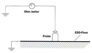
Probe, according to std, with conductive rubber is in contact with the surface • diameter 63 mm • weight 2,27 kg
