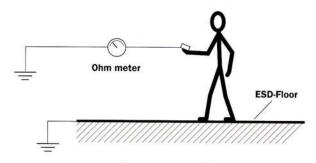
– Ohm meter, like in Pos. 1 – Resistance recommendation between 7,5 x  $10^5~\Omega$  – 3,5 x  $10^7~\Omega$  – ESD-floor is tested with a person standing on it, with ESD-shoes
